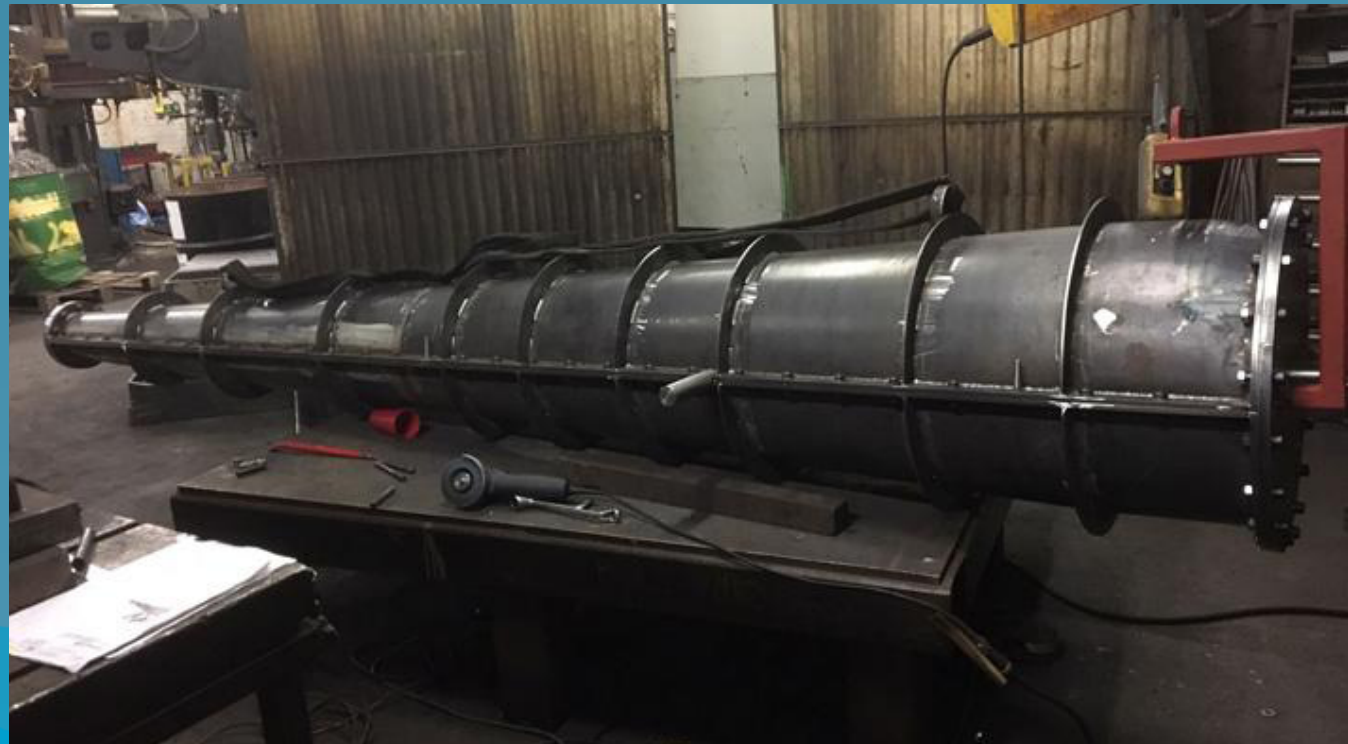
Cast for polyurethane dynamic bend restrictor.
