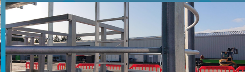
Platform module, showing ladders, gratings and railings. Image courtesy of Hutchinson Engineering. All rights reserved.
