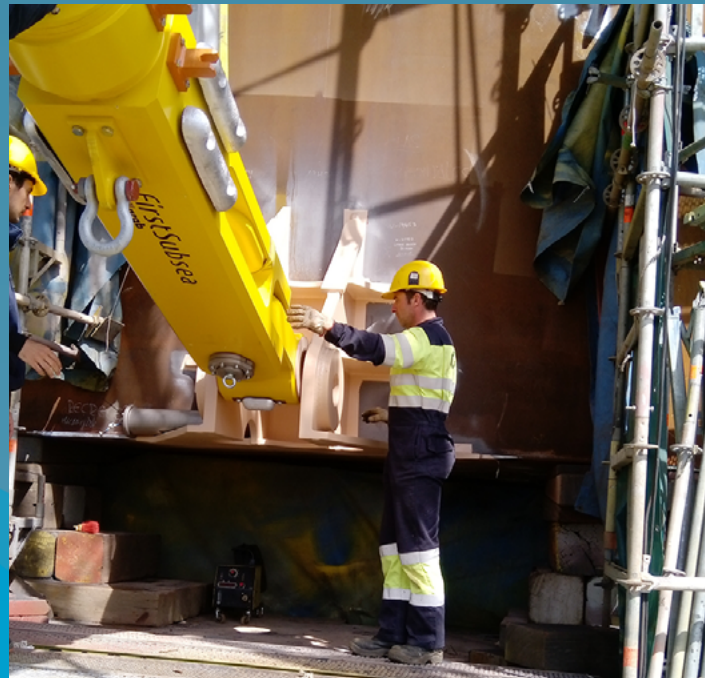
Mooring quick connector assembly. Image courtesy of First Subsea. All rights reserved.
