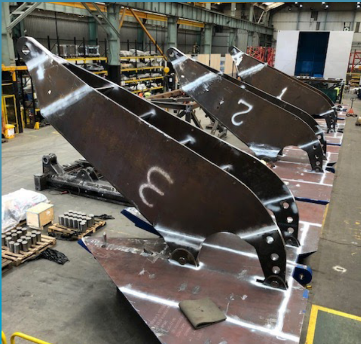
Drag embedment anchor after flat plate welding and weld finishing. Image courtesy of Bruce Anchor. All rights reserved.
